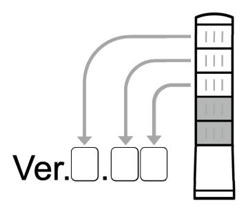
For a detailed verification of the current version, the "REVOLITE EDITOR" application can be used to check from the PC. If the is no personal computer, etc., available in its environment, contact your nearest Patlite Sales Representative and tell them the status of LED tiers displayed to determine the current firmware version.
