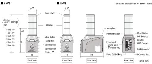
\* Do not use the USB connector as a power supply or for charging
