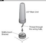
Thread the lead wires through the Multi-mount Bracket and wiring hole, before installing the main unit to the bracket.
