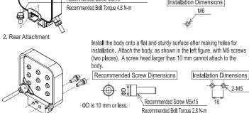
4-3. Fixing of the Adjustment Angle (T Type, PT Type)
